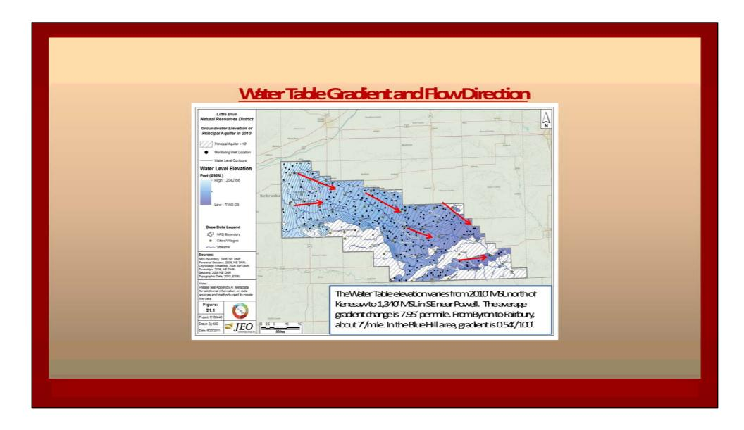
The ground water movement in the saturated sands and gravels is generally from NW to SE across the District. However, the flow direction may be altered by geologic factors, intensive pumping, or recharge. Flow patterns change slightly with each year's conditions and are reflected in annual static groundwater level readings. The natural flow movement through the saturated sands and gravels of the District is approximately 300' to 400'/ year when not influenced by water well pumping.
