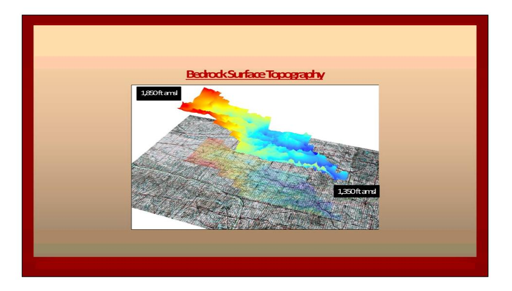
An easier way to visualize the irregularities of the bedrock formations is to project the bedrock elevations in a three dimensional view. Note the peaks and valleys throughout the range. The peaks shown reflect some geologic high points called "bedrock highs" where the overburden may be thinner. The valleys reflect the deepest pockets where the overburden containing saturated sands and gravels are their thickest. Now lets look at the material that lies above the bedrock.
