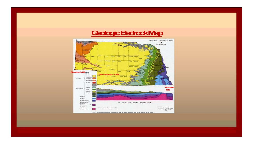
At the base of most test holes is the geologic bedrock formations. The bedrock layers of the earth are laid one on top of another like stacked plates which have had the edge sheered off as you move from west to east across Nebraska. The highest bedrock elevations are found in the western part of the State and the lowest elevations in Southeastern Nebraska.
