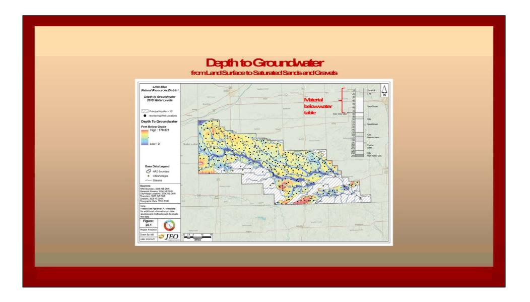
One geologic component which affects water quality from nitrates is the depth to water from the land surface. Those areas having the thickest over-burden and greatest depth to the water table provide a higher level of protection to the aquifer over time. Those areas shown in blue and bluish tints indicate the most vulnerable locations because of thinner overburden and/or higher water tables.
