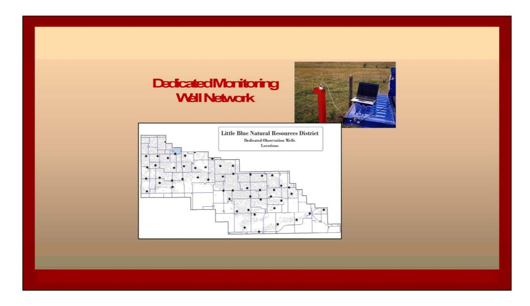
The District also maintains a dedicated monitoring well network containing 50 wells, each equipped with a continuous data logger capable of providing two or more water table readings daily. This network has been invaluable in assessing the impacts of well pumping, the recovery time of each well and the role that various geologic characteristics play in water availability across the District.
