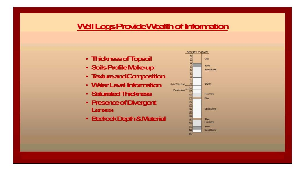
These test hole logs and well logs provide information about the thickness and makeup of soils, texture and composition of the materials, water level information and saturated thickness of the aquifer, the presence of divergent or impermeable lenses and the depth and type of bedrock that underlies the site. It is interesting to note that no two test holes or well logs are exactly identical and many have extensive variability.
