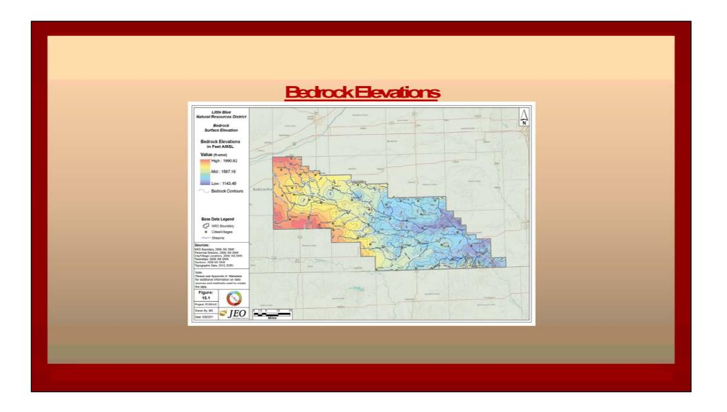
But the surface of the geologic bedrock formations are not a level plain as some might imagine. This map shows the geologic bedrock elevation contours and depicts various hills and valleys that are present across the top of the bedrock layers, much like you see contours on the land's surface.
