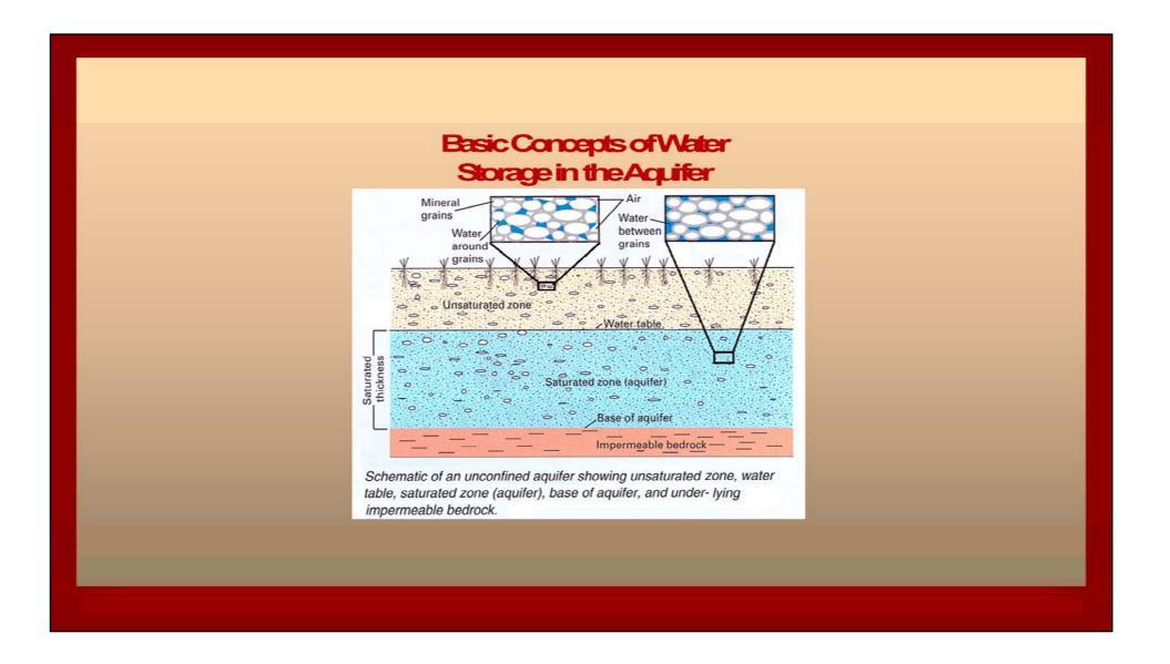
In the environment, we typically find the unsaturated zone, above the water table, and the saturated zone, that which lies below the normal water table. Water is in constant motion, albeit very slowly, as it migrates from the land surface to the water table, and through the water table laterally from areas of higher elevation to lower elevation.
