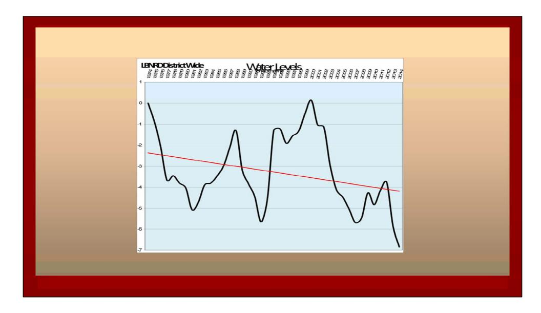
This chart is an ongoing compilation of average spring water table readings which began in 1974. The red line shows a computer generated trend line for the 40-year period. One can see that this chart shows a little over 7' of total aquifer decline in the 40 years of NRD static water level records
