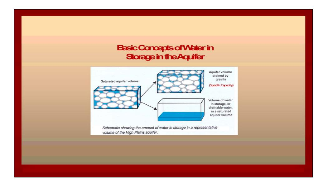
The soils above the water table, typically develop airspaces as water drains from them by gravity. The water which can drain naturally from the soils is referred to as the specific capacity of the soil. In a saturated condition, all the air spaces are filled with water as shown by the block at left. The amount of water which can drain from a saturated soil is dependent on the makeup and texture of the soil materials.
