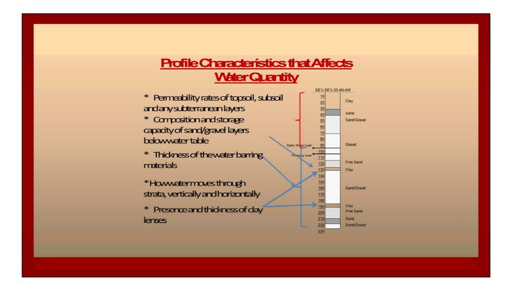
Similar characteristics affect the availability of water. Those factors include: permeability rates and composition of the soils material, thickness of water barring materials, composition of sub-water table materials and the presence of clay lenses or other restrictive features.
