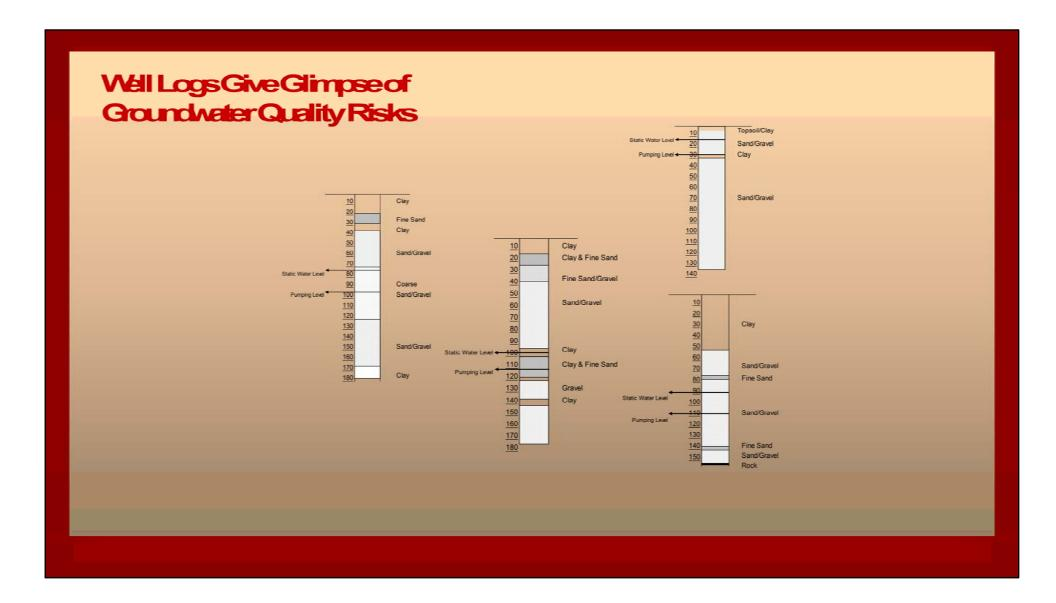
As mentioned earlier, no two well profiles are the same. These actual well driller's logs show varying characteristics and help to assess the risks of groundwater contamination graphically. The more sand that exists above the water table, and the higher the water table, the quicker surface contamination could reach the groundwater below.
