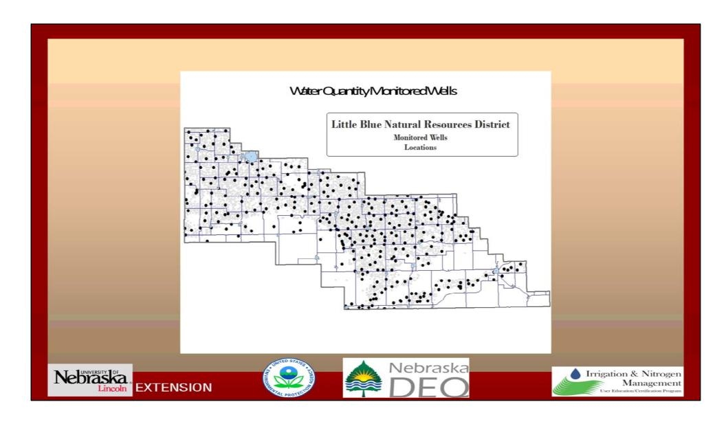
The Little Blue NRD tracks the impact of the development and groundwater uses on the aquifers through a network of 320 irrigation and other wells that are used for biannual static water measurements. These wells give us a picture of the annual fluctuations in the water table, from the impacts of seasonal pumping reflected in our fall readings, to the impacts of groundwater recharge and the ability of the groundwater table to recover through the off season.
