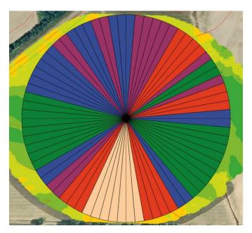
I. <u>Pivot Speed Control Systems</u> guide the pivot system controls to speed up or slow down, depending on specific field conditions, to achieve the desired application rate for each pie shaped section of the pivot's circle.
