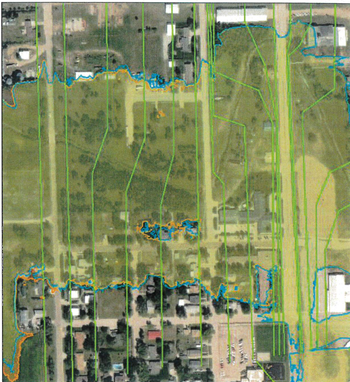
Figure 6. Flood inundation extents with modified channel cross section.
