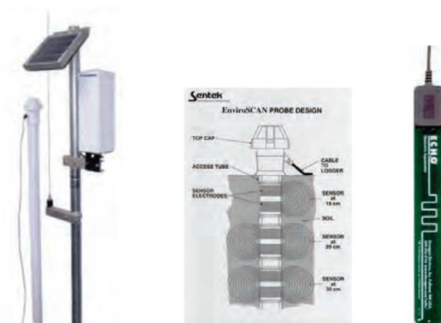
Figure J-8. Examples of the AquaSpy, EnviroSCAN, and ECHO capacitance probes for soil water monitoring.
