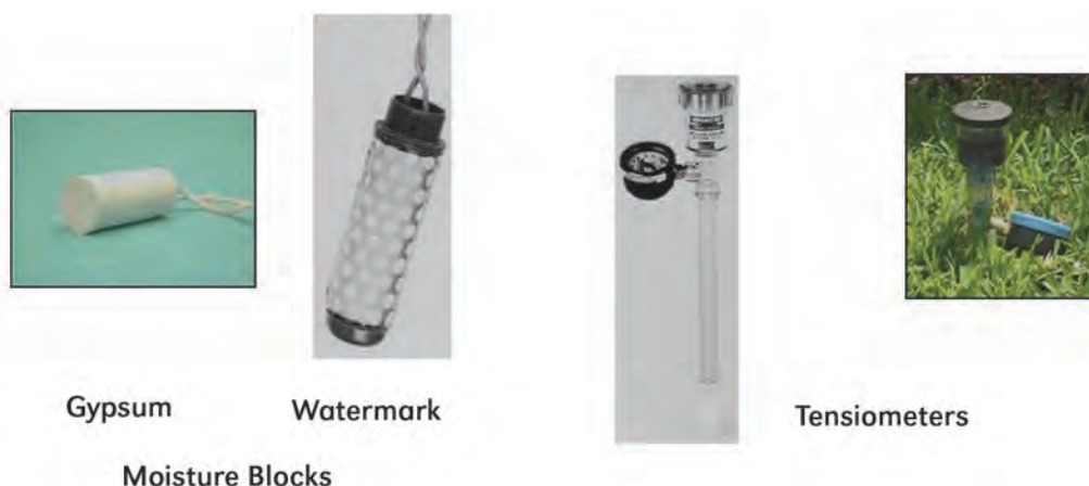
Figure J-4. Methods of measuring the soil matric potential.
