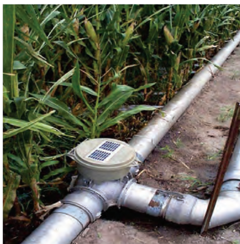
Figure K-5. Typical surge valve installation in the Platte Valley of Nebraska.
