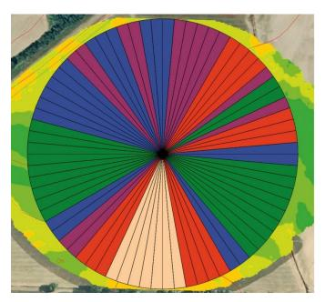
I. <u>Pivot Speed Control Systems</u> guide the pivot system controls to speed up or slow down, depending on specific field conditions, to achieve the desired application rate for each pie shaped section of the pivot's circle.
